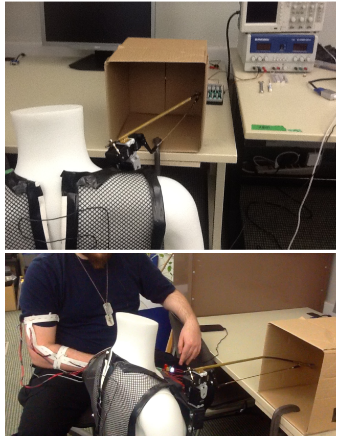
Fig. 2. The experimental setup: a confined workspace, the robotic arm, and an experimental subject with attached vibrotactile feedback sleeve.
