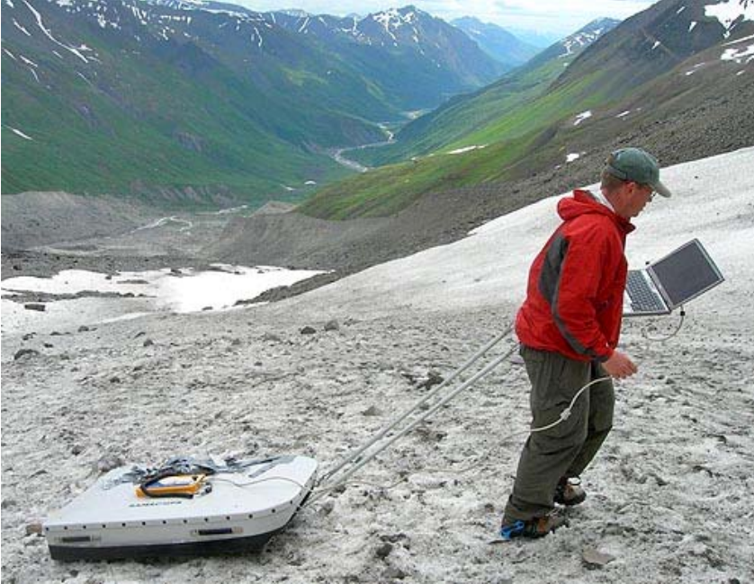
Ramac GPR system mounted in a sled
