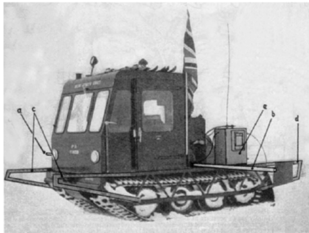
Fig. 1. Muskeg vehicle with separate unipole aerials (a, b) for transmission and reception. The 'Dexion' extensions (c, d), which increased the effective electrical length of the vehicle, were found necessary to reduce the direct coupling between transmitting and receiving aerials and to provide correct electrical loading. The box (e) contains the electronic equipment except for a display unit mounted in the vehicle cab
