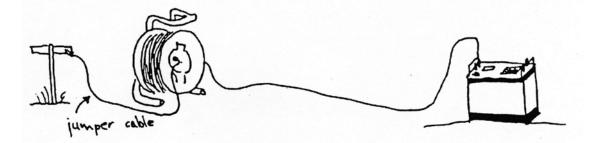
• Reels of wire should not be placed close to the unit, as they act as electromagnets when current flows through the wire.
