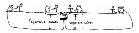
• Cables carrying electric current to current electrodes (A and B) and those detecting voltages at the potential electrodes (M and N) should be separated to avoid cross talk.
