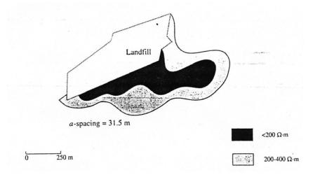
Producing a map like this requires that the 4-electrode Wenner array is moved across a grid of points on the surface. Similar results can be obtained with much less field effort using shallow **electromagnetic** exploration systems (e.g. Geonics EM31 and EM34). These instruments do not require electrodes to be placed in the ground and are essentially large metal detectors. For more details see below and in Geophysics 424.
