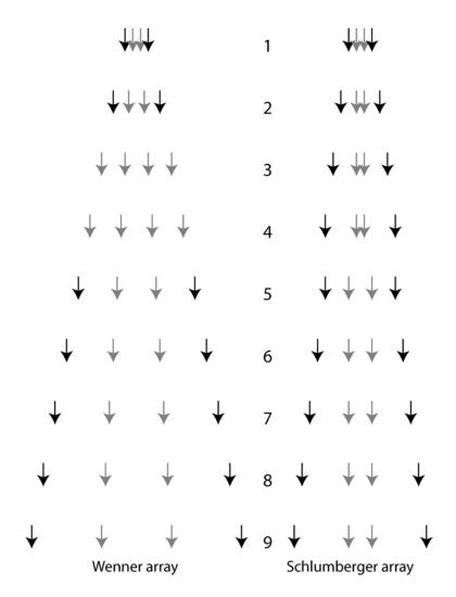
Potential electrodes shown in **grey**, current electrodes in **black**. Note that in the Schlumberger array, the potential electrodes only move at step 5
