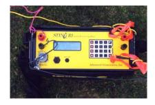
• The electrodes are usually stainless steel stakes. If the surface is very dry, then salt water may need to be poured over the current electrodes (M and N) to lower the contact resistance.
