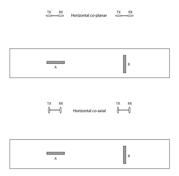
A frequency domain EM survey is flown over two buried conductors. Two configurations of TX and RX are used. Assume that the secondary magnetic field  $(H^S)$  is in phase with the primary magnetic field  $(H^P)$ .
