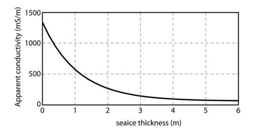
(c) The instrument reading was 600 mS/m. Estimate the ice thickness (D) at this location from the graph you plotted in (b)
