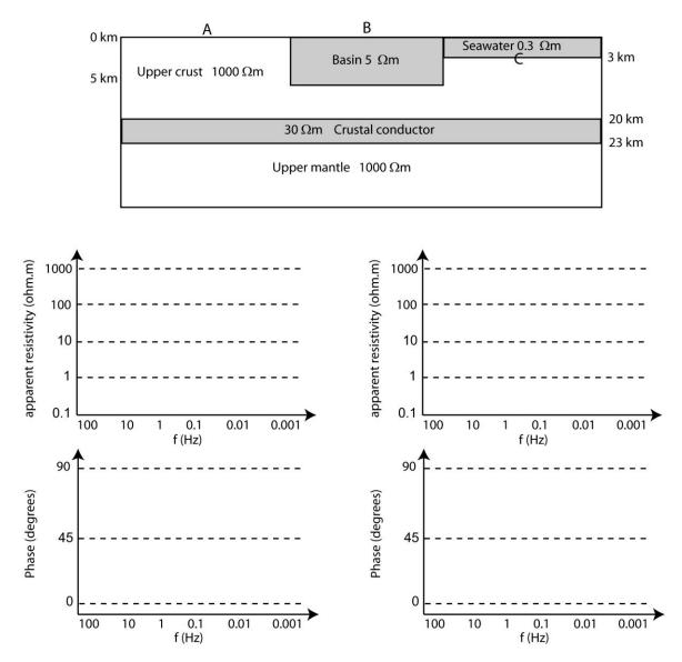
Figure above shows the crustal resistivity structure of a coastal area.
