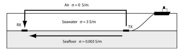
In a marine CSEM survey, the EM signals travel diffusively from transmitter (TX) to receiver (RX) by the **two routes** shown above. In the CSEM survey shown above the seawater depth was 400 m and the transmission frequency was 4 Hz
