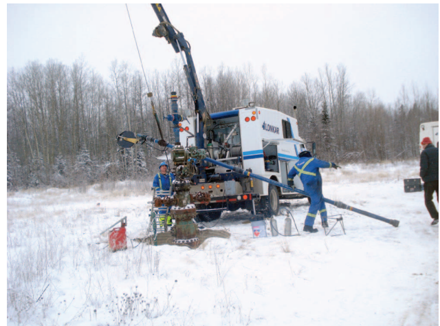
Figure 11. Preparing for temperature logging of the Hunt well after filling the well with water in December 2010.
