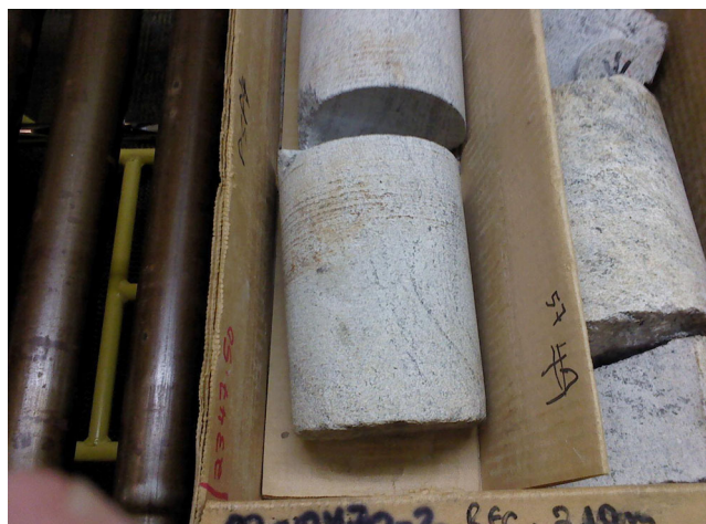
Figure 5. Granitic core from the deepest section of the Hunt Well (below 2300 m). The diameter of the core is 4 inches (10 cm).
