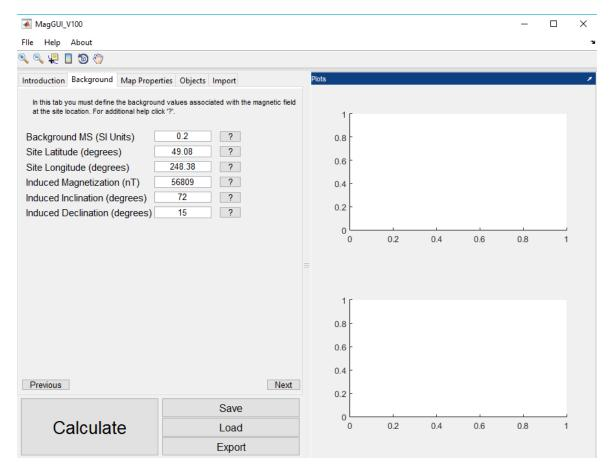
The "Background" tab contains all the inputs required to describe the location of the survey. This includes the site latitude, site longitude, induced magnetization, inclination, and declination.
