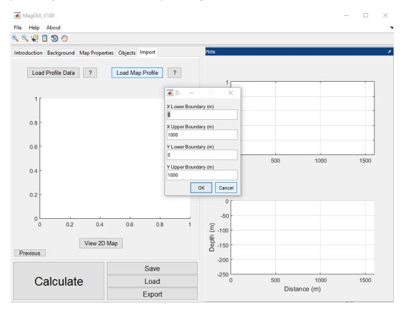
For this tutorial we will input the "X Lower Boundary" and the "Y Lower Boundary" to be 0m. The "X Upper Boundary" and the "Y Upper Boundary" is inputted as 1000m. Click "Ok" and choose the appropriate file to load, in this case MapExample3.xls.
