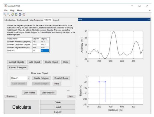
To close the polygon the last vertex can either overlap with the first vertex or the user can double click.
