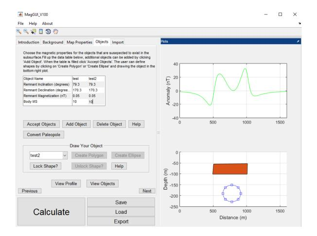
In the "Objects" tab the user is required to create the magnetic objects responsible for a magnetic anomaly. The user does this by inputing the proper remnant magnetization data for their object(s) into the data table. **The name for each individual object must be unique.**
