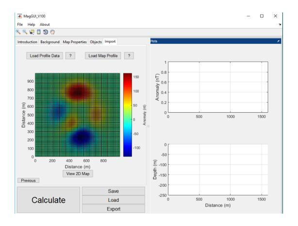
The user clicks and drags across the map profile to get a magnetic anomaly plotted into the profile plot (top plot). If you want S-N profile, the first point on the profile should be the most southern point. Then move the line towards the North. The X-Offset from North will be 0°. If you move your profile from the north to the south (The X-Offset from North will be 180°), then 'drag' the line from the north to the south.
