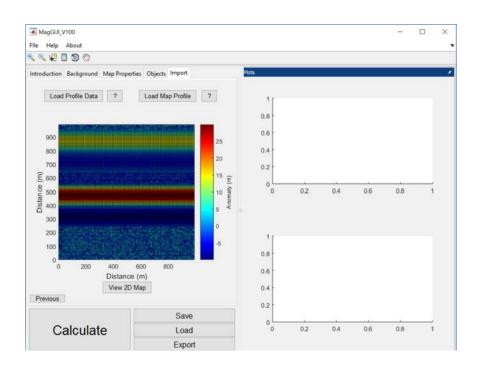
The user then drags a line across the profile. In MapExample3.xls we see that there are 2 symmetric objects in the E-W direction, therefore the most useful profile may be an S-N profile as shown below.
