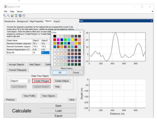
Once the colour has been select the mouse cursor is brought to the bottom right plotting area where a crosshair should be visible.
