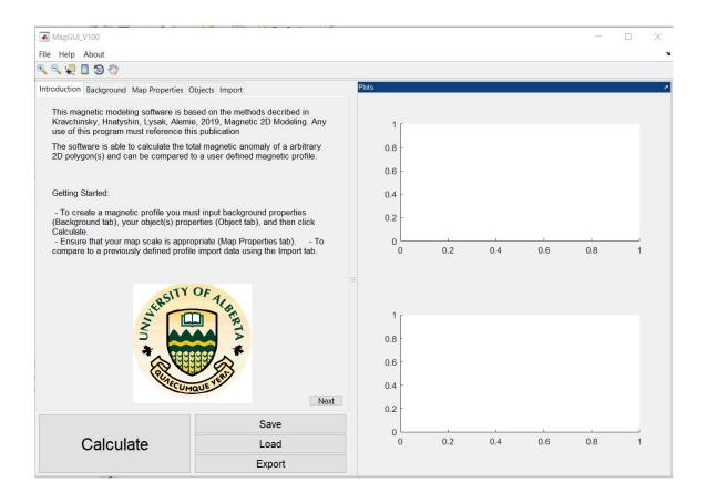
MagMod V1.00 is divided into separate tabs into two section. The left side contains the Introduction, Background, Map Properties, Options, and Import tabs. While the right side contains plots associated with magnetic profiles and the subsurface.
