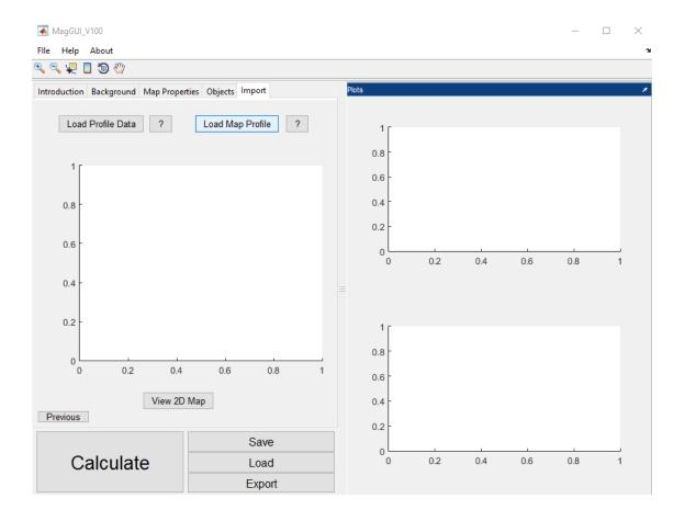
The "Import" tab allows the user to either load a 2D magnetic profile ("Load Profile Data") into the profile plot or to load a magnetic anomaly map ("Load Map Profile") from which a profile can be created. These profiles must be in a .xls or .xyz format using UTM coordinates (use example spreadsheets as a template or see the figures below) to be loaded properly.
