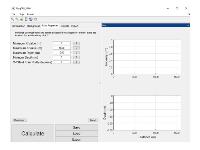
The "Map Properties" table sets the domain for the profile used in MagMod. Any imported profile will automatically update the "Minimum X-Value", "Maximum X-Value". Map profiles will also adjust the "X-Offset from North" value to the orientation of the loaded profile
