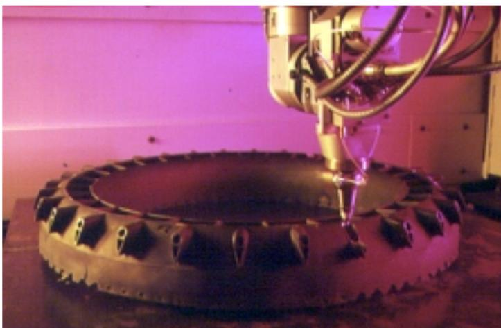
3D laser cutting for difficult-to-machine aerospace component was successfully applied
