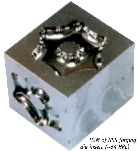
HSM of HSS forging die insert (~64 HRC)
