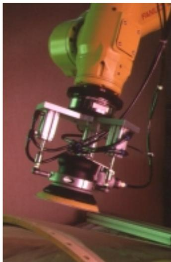
*The compliance-controlled robotic system enhances aircraft canopy polishing*
