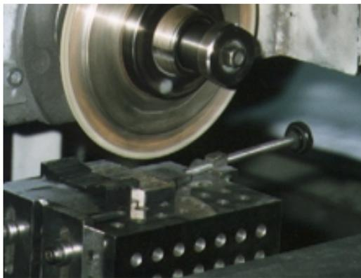
*Profile grinding of a sample with GrindStar*
