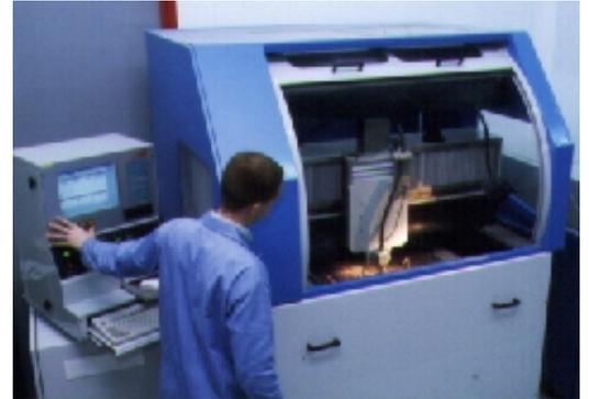
*Precision abrasive water-jet cutting system*
