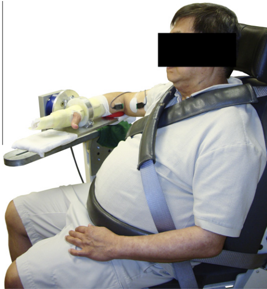
Fig. 1. Image of the experimental setup with the paretic arm in the test configuration. The metal forearm interface plate and ring are mounted directly to a 6-DOF load cell. A delrin interface ring connects the wrist of the test subject with a fiberglass cast to the metal ring. EMG recording and stimulating electrodes are placed over the biceps brachii muscle.
