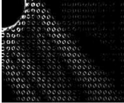
Figure 4. Pattern of internal waves generated by an oscillating cylinder, in the upper left-hand corner, as visualized by qualitative synthetic schlieren applied to a pattern of equally spaced dots behind the tank. Adapted from Figure 7c of Dalziel et al. [2000].
