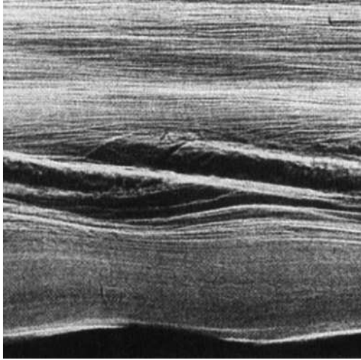
Figure 1. Internal wave breaking near a critical layer as visualized by shadowgraph. Extracted from Figure 7 of Koop and McGee [1986].
