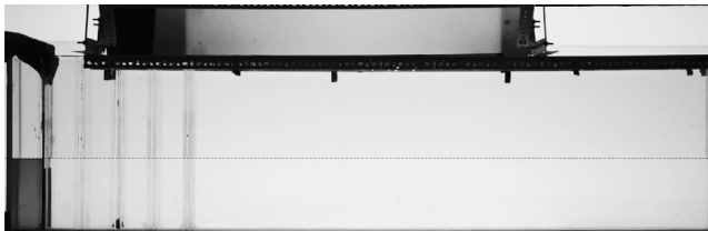
FIG. 1. Snapshot from an experiment just before gate is extracted. For this experiment the dyed lock fluid is 99.2% glycerol situated in a lock of width \ell = 8.3 cm. The ambient fluid to the right of the gate is fresh water (the superimposed dashed line indicates its surface). The height of both lock and ambient fluids is 19.9 cm. The angled mirror above the tank gives top views of the ensuing flow between approximately 50 and 130 cm from the left end of the tank.
