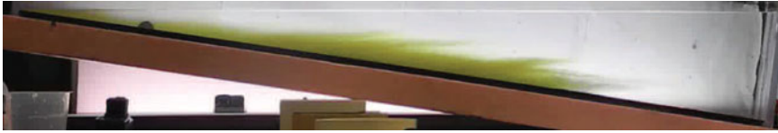
FIGURE 5. (Colour online) A snapshot from the same experiment shown in figures 3 and 4(c) but taken at a time well after the current has separated from the slope. Several fingers of dye are evident emanating horizontally into the stratified ambient along the length of the slope.
