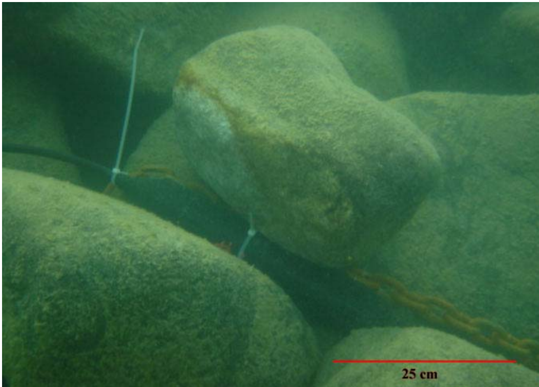
Figure 4-2) Placement of the 4-C sensor. The sensor is attached to the chain and also placed under rocks to ensure coupling.
