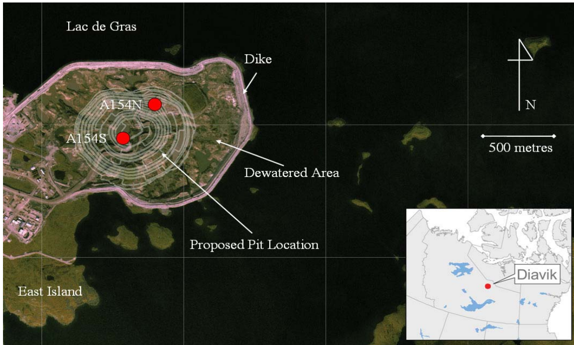
Figure 1-1) Air photo showing the proposed pit (A154) location within the drained area near East Island on Lac de Gras. The A154N and A154S kimberlitic pipes are indicated in red. The inset map shows the location of DDMI in Canada's Northwest Territories. Courtesy, DDMI.
