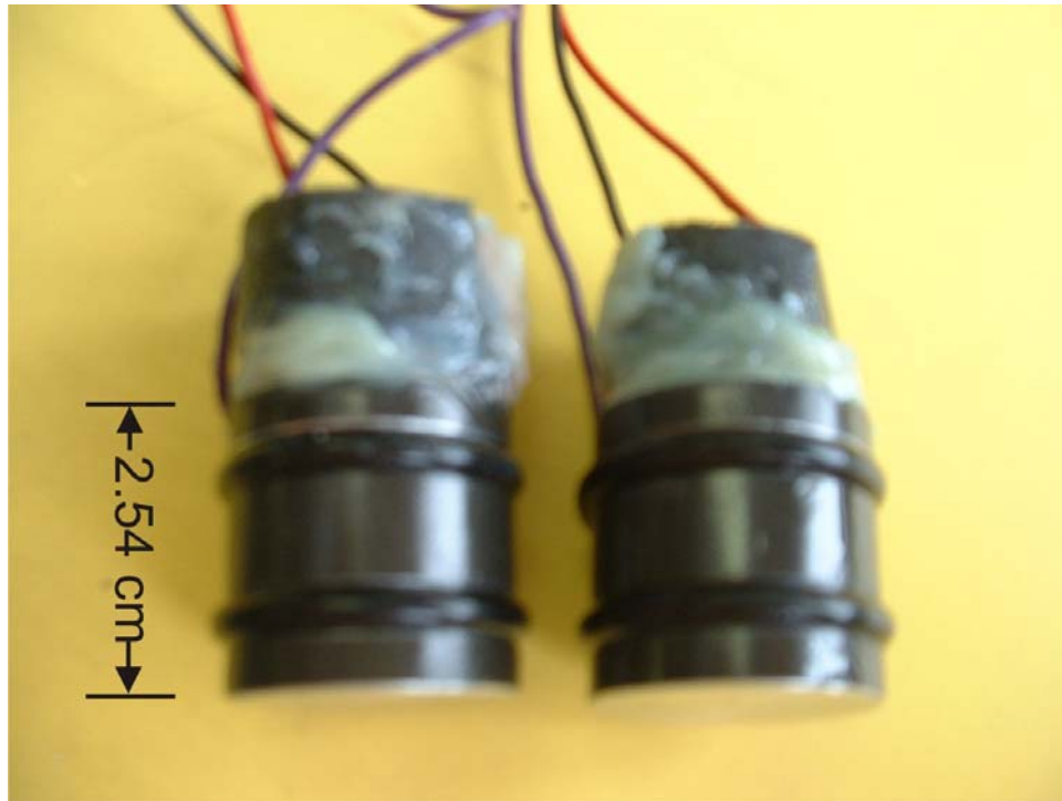
Figure 3.2 - Photograph of the finished transducers. The piezoelectric ceramics are buried in the urethane rubber on the top of the aluminum buffers as shown in Figure 3.1.
