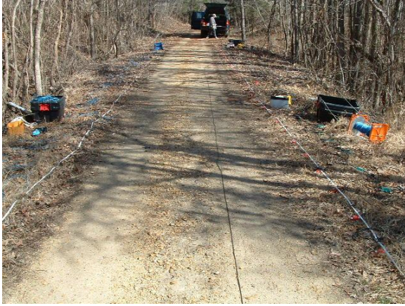
Figure A-11 this is the surface layout of tunnel 5, on the left is the ERT survey, the right is the seismic
