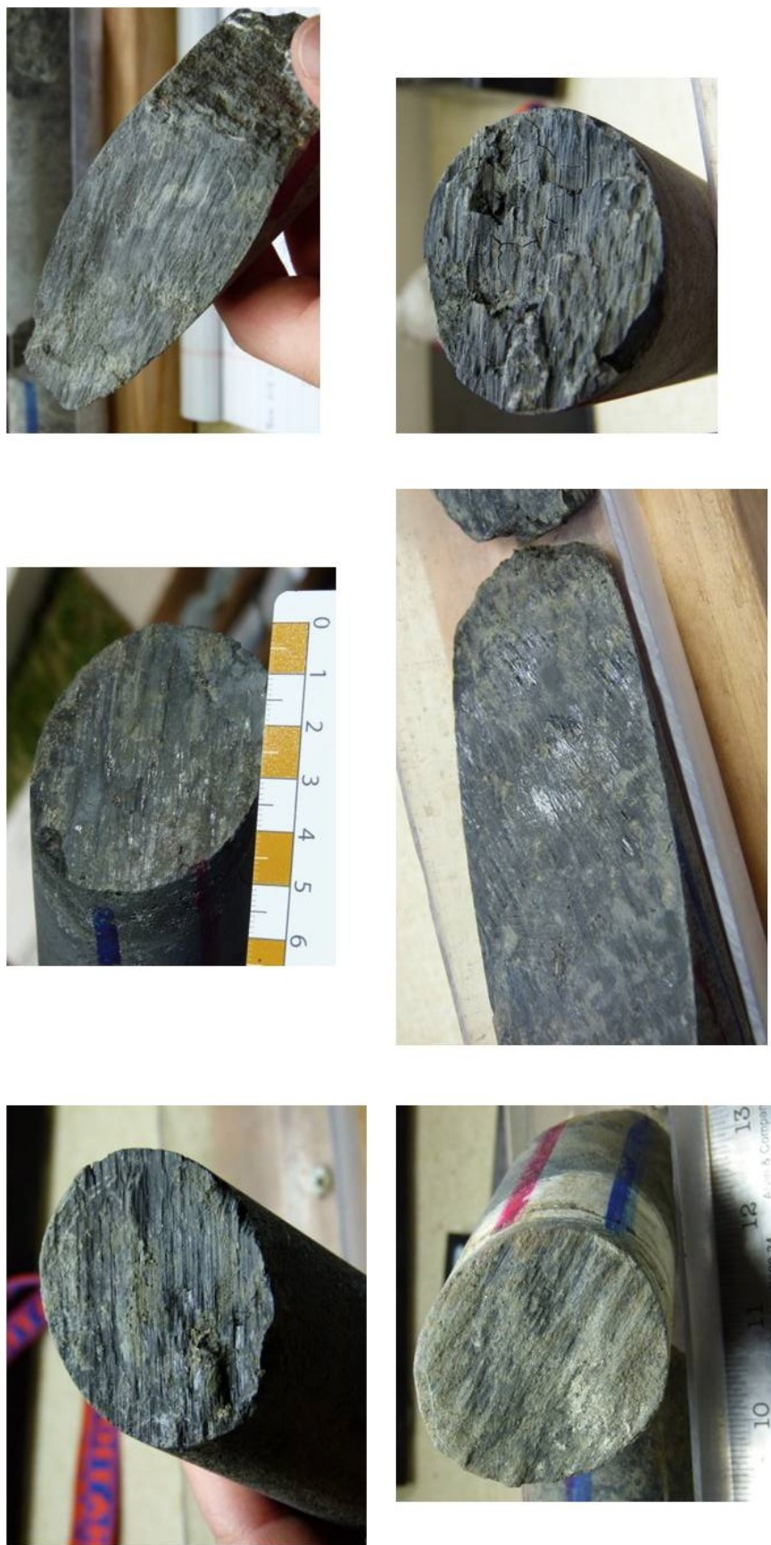
Figure 4-7. Examples of structural and mineral slickenlines in the MH-2 core
