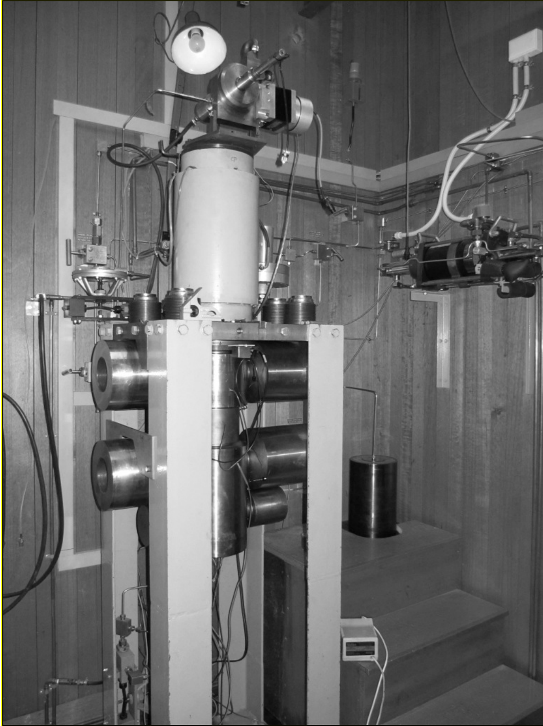
Figure 2.2: Forced oscillation pressure vessel at Australian National University for 0.001-1 Hz shear and Young's modulus measurements.
