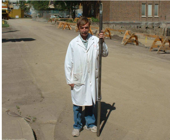
Figure 1.11: The detector consisted of a 3 component SIE wall locking geophone package.
