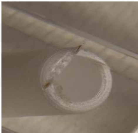
Figure 3.13 A closer view of the bottom hole fractures for Sample #3.
