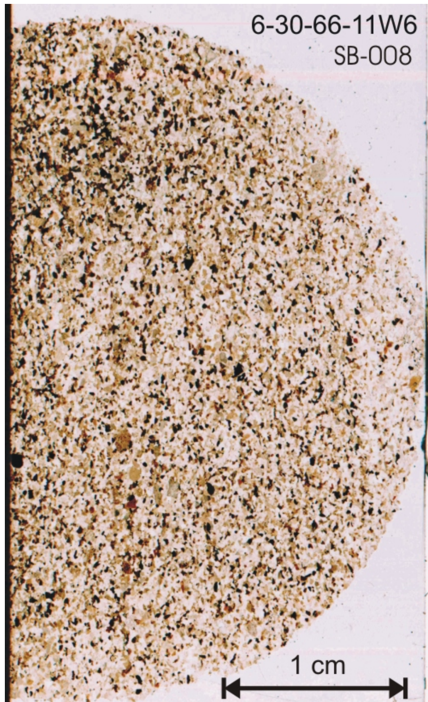
Figure 4.4: Thin section of Cadotte sandstone sample SB008 (depth of 2455.1 m in 15-29-66-11W6).
