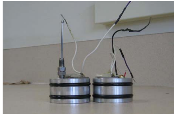
Figure 3.4: A pair of buffers attached with P- and S-wave transducers using conductive epoxy.
