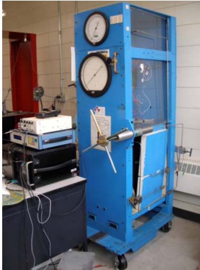
Figure 6.3 Pressure vessel, pulser and oscilloscope
