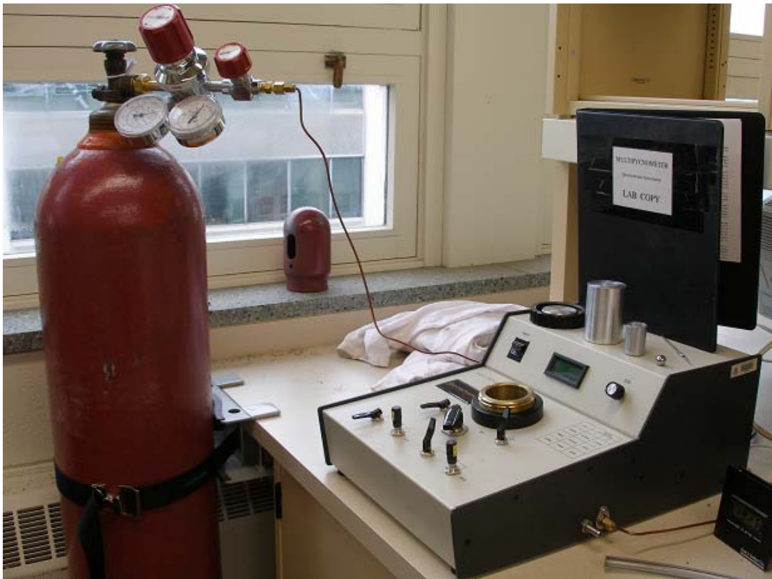
Figure 7.11 Helium Multipycnometer (by Quantchrome Instruments, model # MVP-D160-E) for grain density measurement
