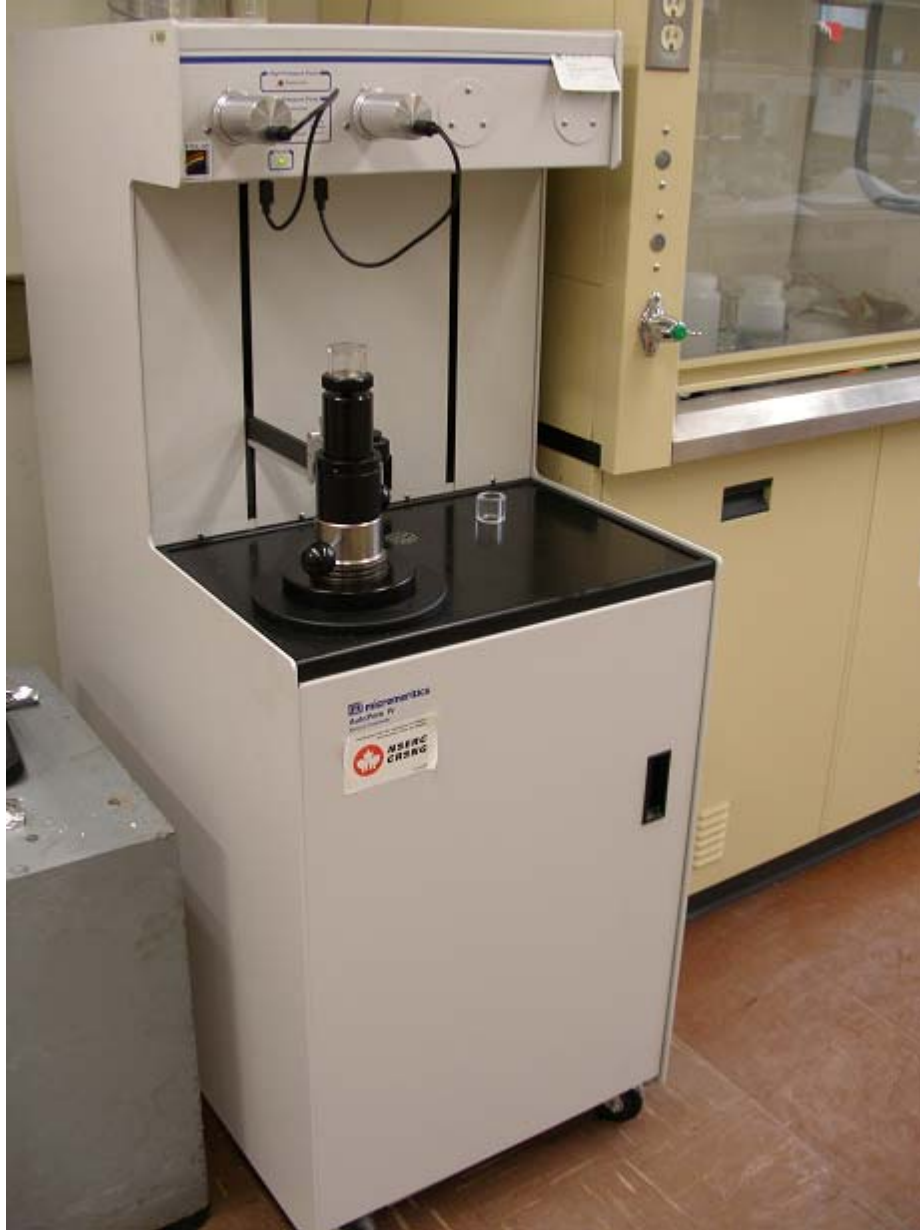
Figure 7.8 Mercury porosimeter (AutoPore IV ® by Micromeritics ® )
