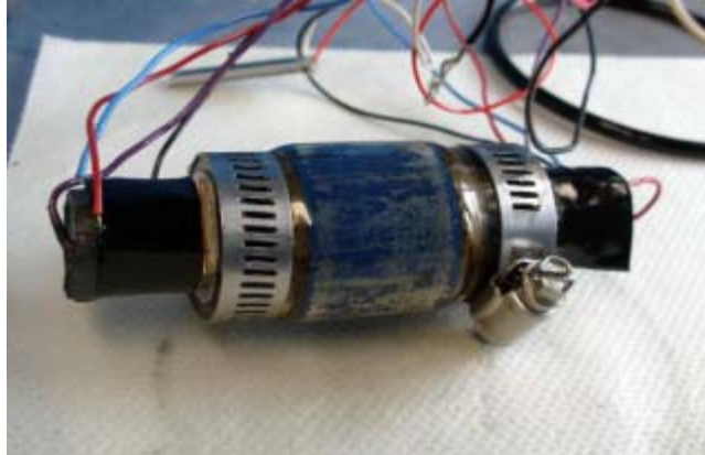
Figure 6.8 Conventional preparation of test samples (with P and S wave transducers stacked)
