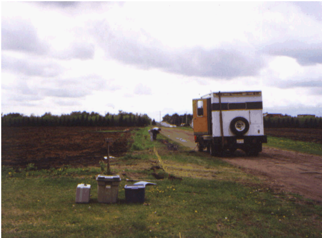
Figure 3.3: Seismic recording truck next to the receiver line at the Edmonton Research Station.
