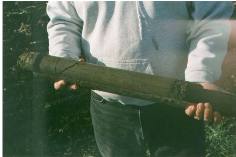
Figure 4.3: A soil core taken using a split spoon sampler.
