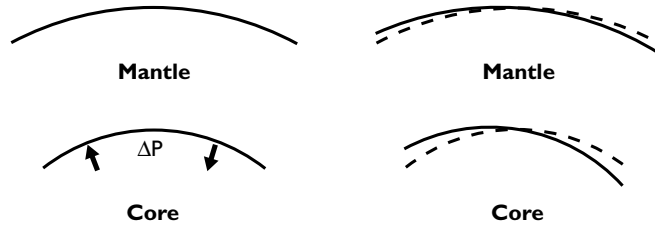
Figure 3.2: Horizontal gradients in pressure at the CMB (left), lead to a radial deformation of the CMB and the exterior surface (right).
