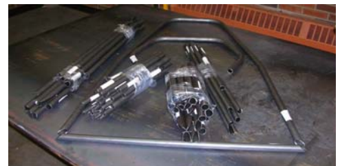
Freshly Cut Chassis Tubes from Marl Technologies
