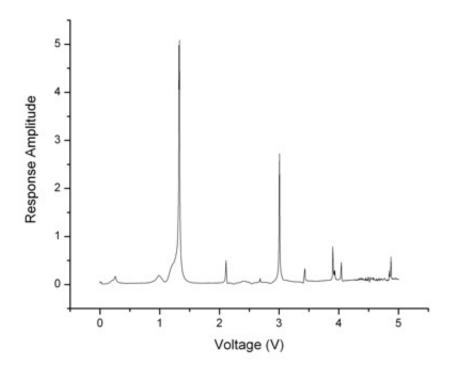
iii) Now it is time to carefully measure the frequencies of as many modes as you can access (limited by the 200 kHz max. operating frequency of the lockin), by determining the frequencies at which the amplitude of response is a maximum for each mode. You can do this either by carefully adjusting the F34 frequency dial by hand (the smaller inside knob allows finer adjustments) and/or by setting the frequency below the resonance and then sweeping www.phys.ualberta.ca/cwiki/index.php?...
