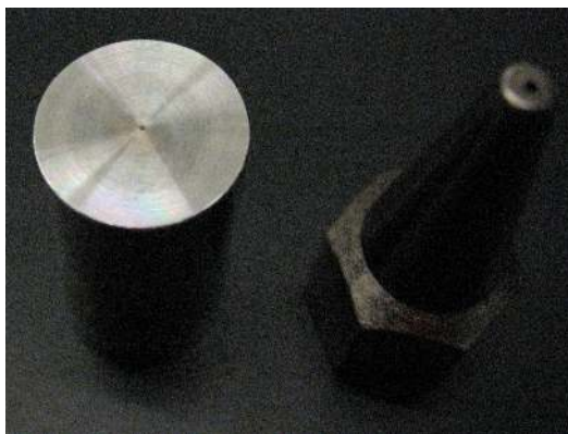
Figure 2.2: Custom torch head with 0.13 mm inner diameter hole (left) and previous torch head with 0.40 mm inner diameter (right)
