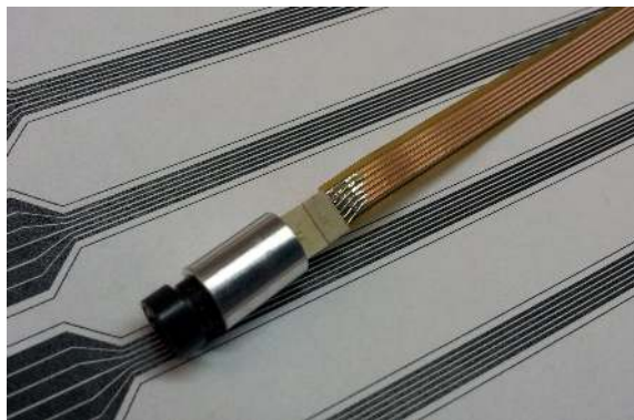
Figure 3.12: Vacuum compatible 3.4 mm CCD camera wired to a custom ribbon cable with a PEEK intermediary connector.
