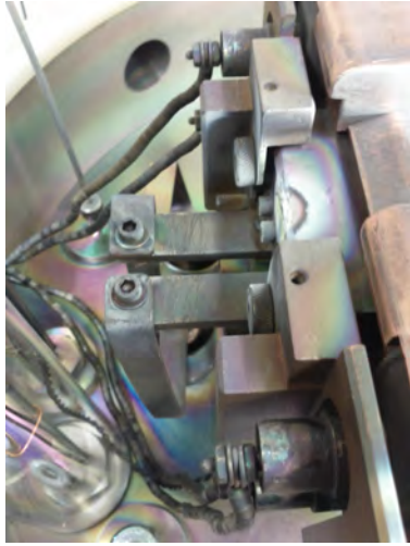
(a) The two electrodes of the e-gun.
