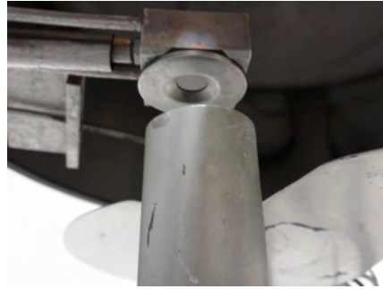
(b) Guide tube to the quartz crystal monitor used to monitor thermal deposition.
