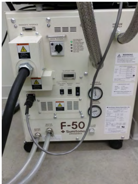
(c) Front view of the compressor for ^3\text{He}/^4\text{He} fridge.
