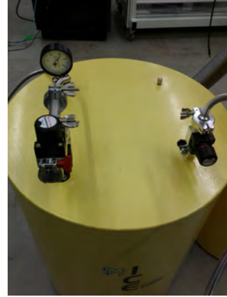
(b) The dump used as buffer to store ^4\text{He} gas outside of the main body of \text{DRYICE}^{4\text{TL}} System.
