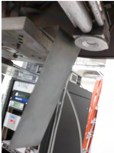
(a) The quartz crystal monitor installed at the same level of the substrate holder to monitor e-gun deposition.
