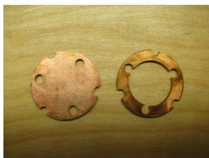
(a) The piece on the left side is a copper substrate made for the sample stage used in ^3\text{He} dipper fridge. The three clearance holes are for substrate mounting, and the dents on the edges were designed for the convenience of running wires through. The piece on the right side by the substrate is a washer used to mount the substrate onto the sample stage.
