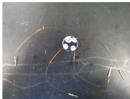
(b) A sample film with four striped copper wires attached to it as leads to take resistance measurements. The wires were glued to the substrate with silver paint and then stycast epoxy for reinforcement of strength. On the other end of each copper wire was a quick connector soldered to it for the convenience of changing sample.
