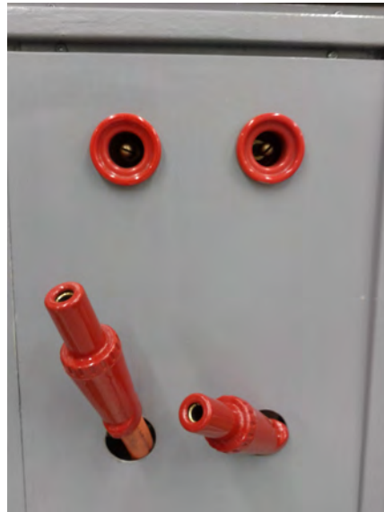
(d) The two electrodes outside the vacuum chamber for thermal deposition.
