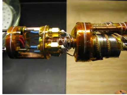
(b) The sample stage is directly connected to ^3\text{He} pot on the probe through a copper support piece.
