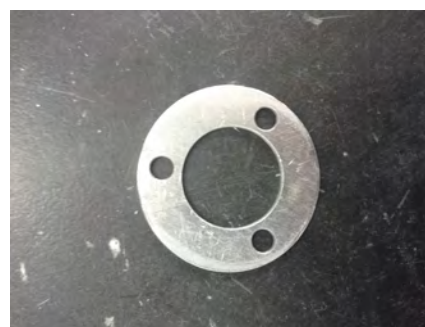
(b) The mask used on top of substrates during depositions to restrict the size and position of the area on where the sample film would be deposited.
