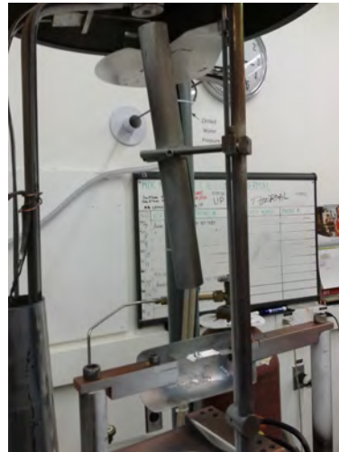
(b) The stainless steel tube used to guide the vapour to the quartz monitor for thermal deposition system.
