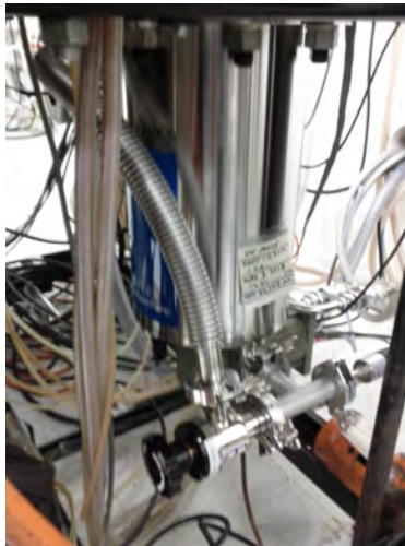
Figure 2.4: The CTI cryo pump used to pump on the vacuum chamber used in depositions.
