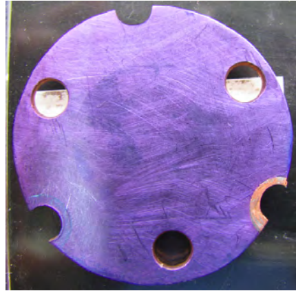
(b) The copper substrate with an adhesion layer of titanium deposited on it.
