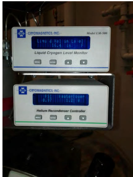
(d) Front view of the helium level monitor (top) and pressure monitor (bottom) for the ^4\text{He} dipper fridge.
