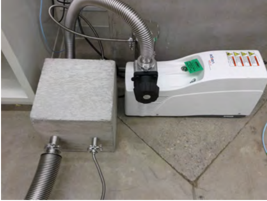
(a) The external pump used on VTI.
