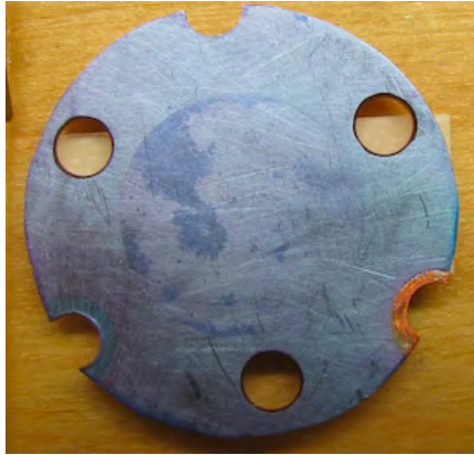
(a) The copper substrate with an adhesion layer of chrome deposited on it.
