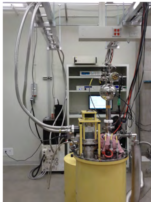
(d) ^3\text{He} probe in the VTI sample space of the ^3\text{He}/^4\text{He} fridge.
