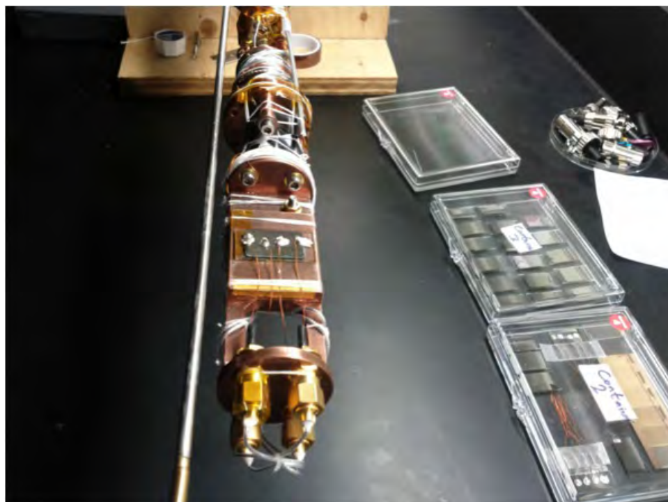
(b) Front view of the sample stage for ^4\text{He} dipper fridge.
