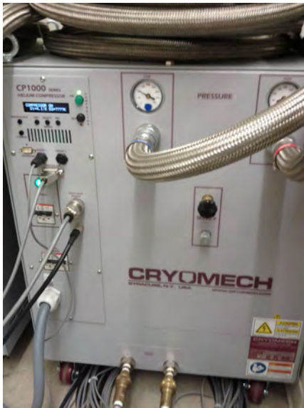
(c) Front view of the compressor for the ^4\text{He} dipper fridge.
