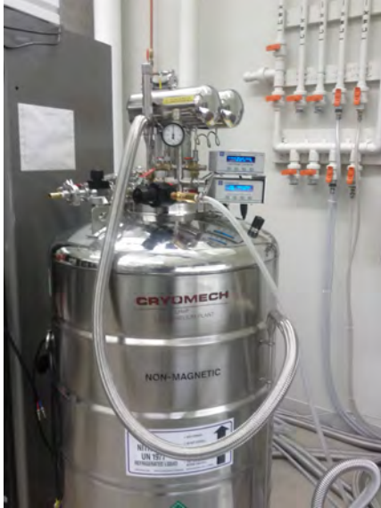
(a) Front view of the dewar of the ^4\text{He} dipper fridge.
