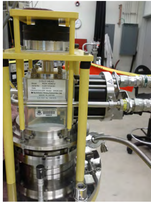
(b) ^4\text{He} condenser located on top of the OVC of ^3\text{He}/^4\text{He} fridge.
