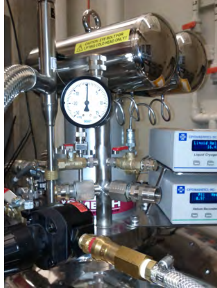
(b) ^4\text{He} condenser located on top of the dewar of the ^4\text{He} dipper fridge.
