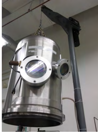
(b) The lifting system for the bell jar.
