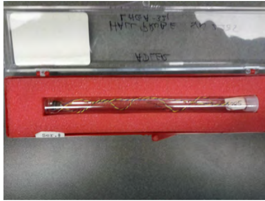
(a) The LHGA-321 hall probe used in our experiments, manufactured by Lakeshore ® , can take measurement of magnetic field at a large temperature range between 1.5 K to 370 K.
