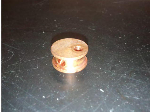
Figure A.1: The bobbin in which a thermometer is mounted.
