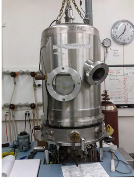
(c) A photo of the vacuum chamber used for both e-gun and thermal depositions.
