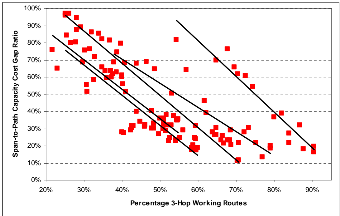
Figure 9.23 – Scatter plot of the gap ratios of NISR-S SCA capacity costs versus the percentage of working routes of three hops or shorter for all 124 test case networks.
