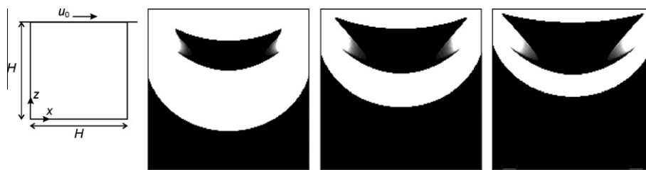
Fig. A3. Lid-driven cavity flow as defined in the left panel. The contour plots are for Bn = 5, 20, and 50 (left to right). Black indicates \dot{\gamma} = 0 (i.e. unyielded); white indicates \dot{\gamma} \geq 0.01u_0/H ; the in-between grey scale is linear. Re = 0.05 .
