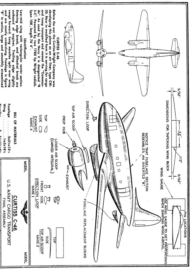
with pilots' cockpit faired into nose. Tapered tailplane with large bulged tabs and rounded tips.
