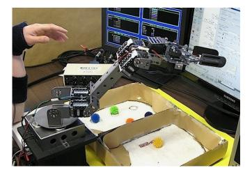
Figure 8. The myoelectric training tool (MTT), a multi-joint robotic prosthesis used to train new amputees.
