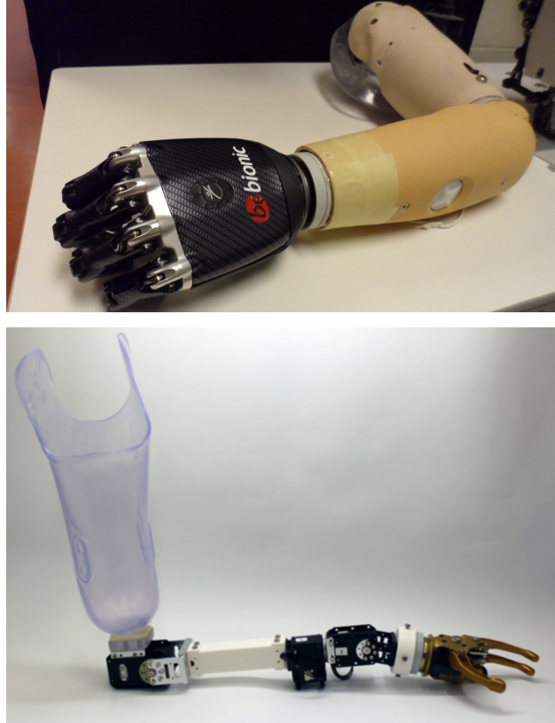
Figure 4.1: Augmentative and restorative prosthetics are of specific interest for incrementally integrating AI into a robotic setting. Top : commercial limb system prescribed to an amputee for use during daily life. Bottom : research robot limb system with direct access to a rich sensorimotor stream (Dawson et al., 2014).
