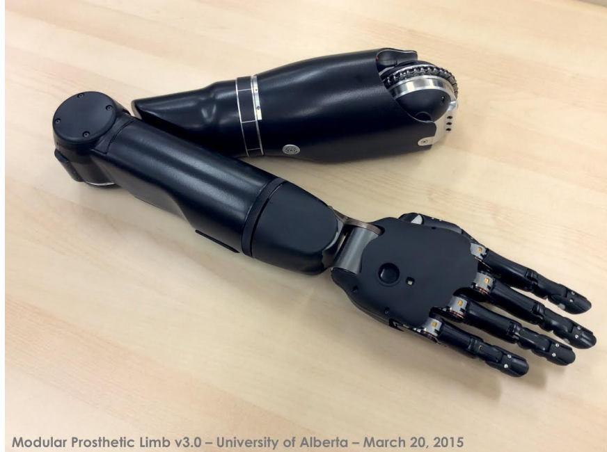
Figure 2.1: The Modular Prosthetic Limb developed by Johns Hopkins University as part of the Revolutionize Prosthetics project funded by DARPA
