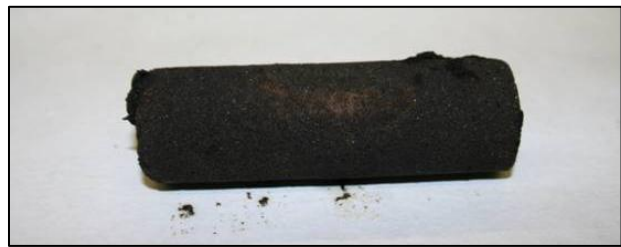
Figure 13: Powder like substance observed at the end of experiments. It is believed that it is clay+asphaltinic components formed during Phase 2.
