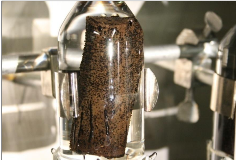
Figure 8: Tiny droplets of oil adhere to the surface of the rock; they are too small to coalesce and overcome adhesion forces.
