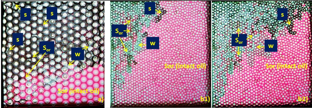
Figure 6-20: Permeability effects on S_{or} during lateral expansion of steam chamber: (a) 3 mm model (2 hours), (b1) 1 mm model (2 hours) and (b2) 1 mm model (7 hours). (s: steam, w: water, o: oil).
