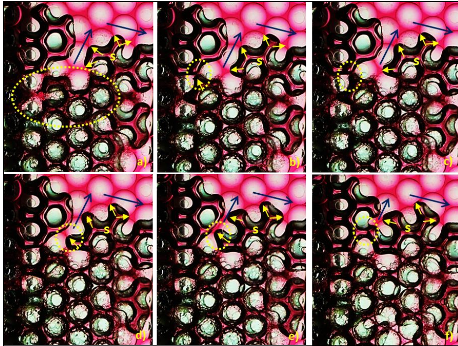
Figure 6-17: Sequence of capillary (hydraulic) continuity lost in the ceiling part of the steam chamber (s: steam).
