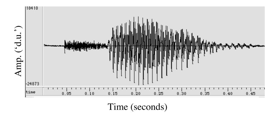
*Note:* Amp. ('d.u.') = amplitude in 'digital units' (proportional to voltage at microphone- scaled by computer hardware)
