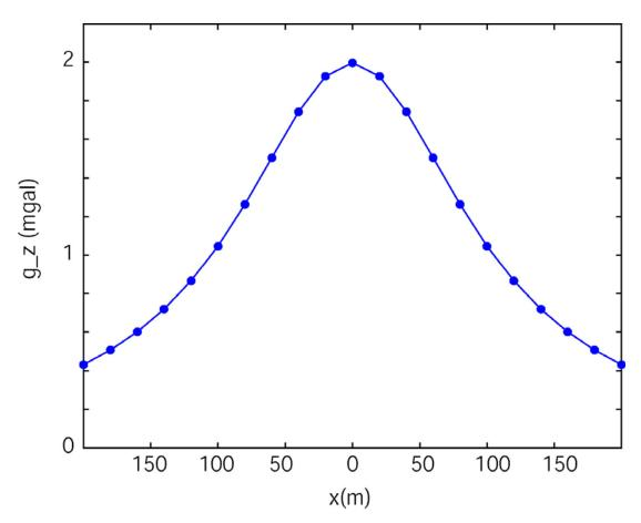
The figure above shows the variation in gravity across an ore deposit that is approximately spherical in shape.
