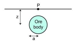
Consider a **spherical ore body** with density  $\rho$  and radius a that is buried at a depth z below the surface. The extra pull of gravity will be greatest at a point P directly above the ore body.
