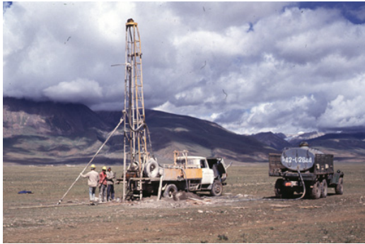
Drilling shot holes in Tibet, 1994
