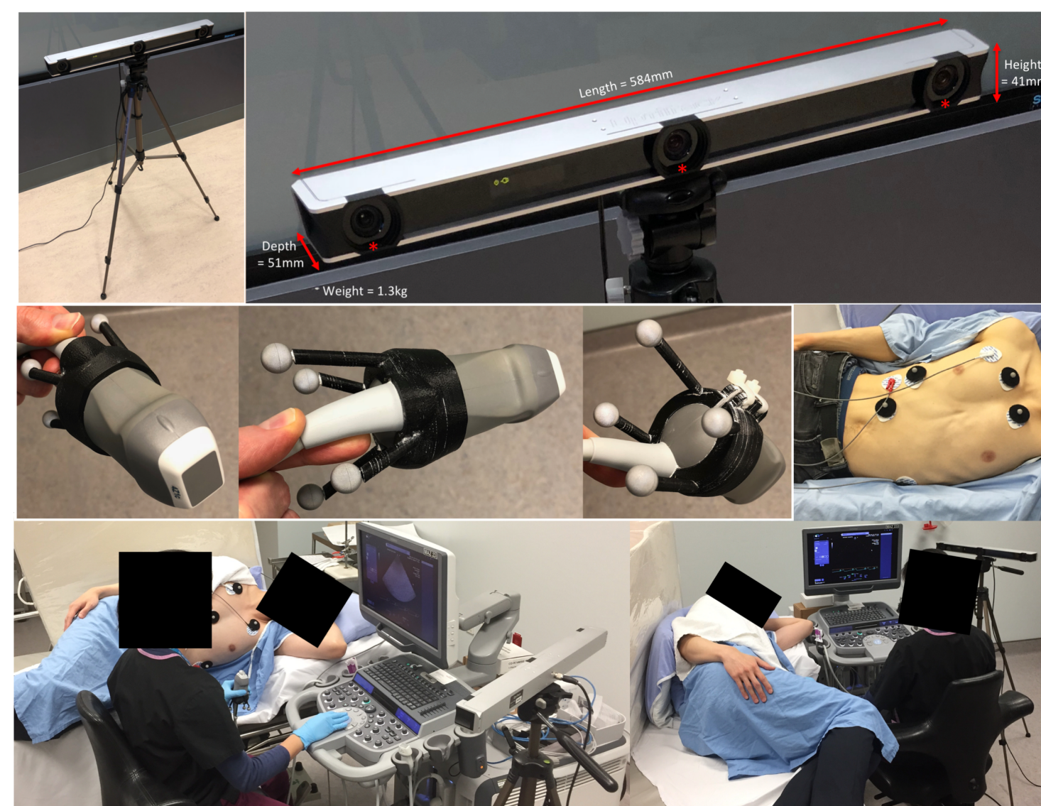
Figure 2: Components of our M3DFE setup. Top row – Optical tracking device. Middle Row – Transducer with mount and markers (left). Note these markers are depicted in red in figures 1 and 4; Chest markers (right). Bottom Row – Relationship between components
