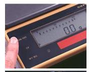
Check if the balance is turned on. If not, press the on/off button and wait until the display reads 0.0 g.
