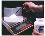
Carefully add substance to the container or paper. Allow the balance to stabilize. Record mass.
