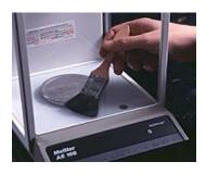
Use the brush provided to clean spills in the weighing chamber. Discard any disposable tare containers, weighing paper, or Kimwipes in the proper waste disposal in the lab.
