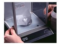
Before recording the mass, close the glass doors and wait until the stability detector lamp goes out. Record mass of solid.
