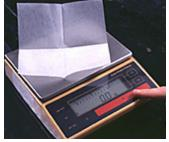
Place a container or large, creased weighing paper on the balance pan. Push tare button to zero the balance.
