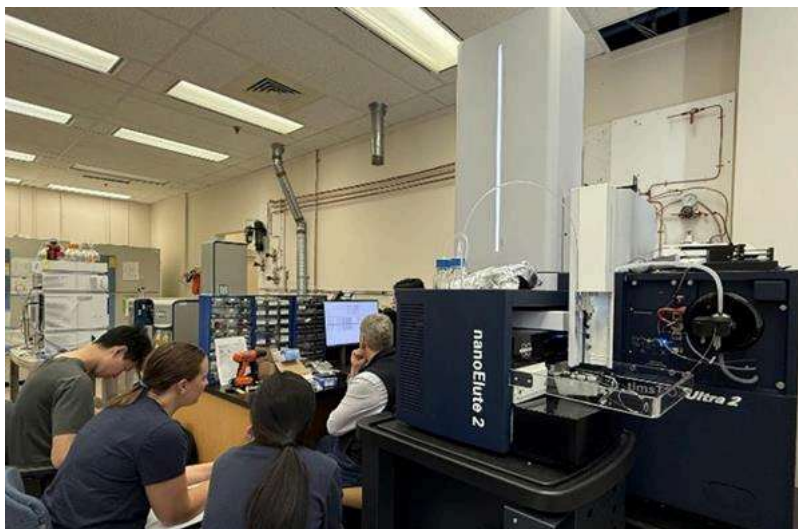
Figure 1. The Bruker timsTOF Ultra 2 mass spectrometry system enables 4D proteomics across the dimensions of liquid chromatography, ion mobility, quadrupole precursor isolation, and time-of-flight analysis of peptide fragments
