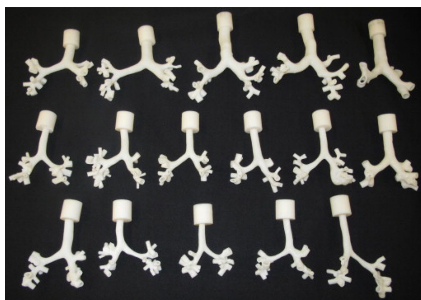
Figure 1. Five realistic adult hollow conducting airway replicas (top row) and 11 child hollow conducting airway replicas (second and third rows). Outer wall thickness is 2mm.
