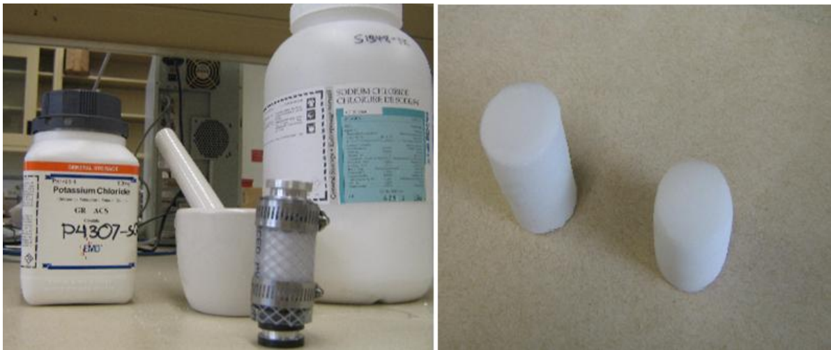
Figure 3-6 Synthetic sample (NaCl and KCl) prepared using cold compressing technique.
