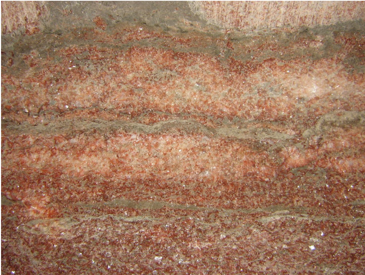
Figure 1-1 Different layers in a Potash mine. The grey colored layers are showing the presence of shale.
