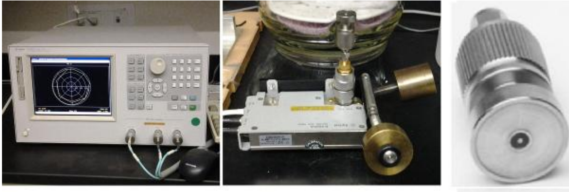
Figure 3-1 Measurement system: Agilent 4991A RF Impedance/Material Analyzer (left), coaxial line sensor (middle), and a magnified picture of the 19 mm diameter sensor (right). Measurements may be obtained over a frequency range of 10 MHz to 3 GHz
