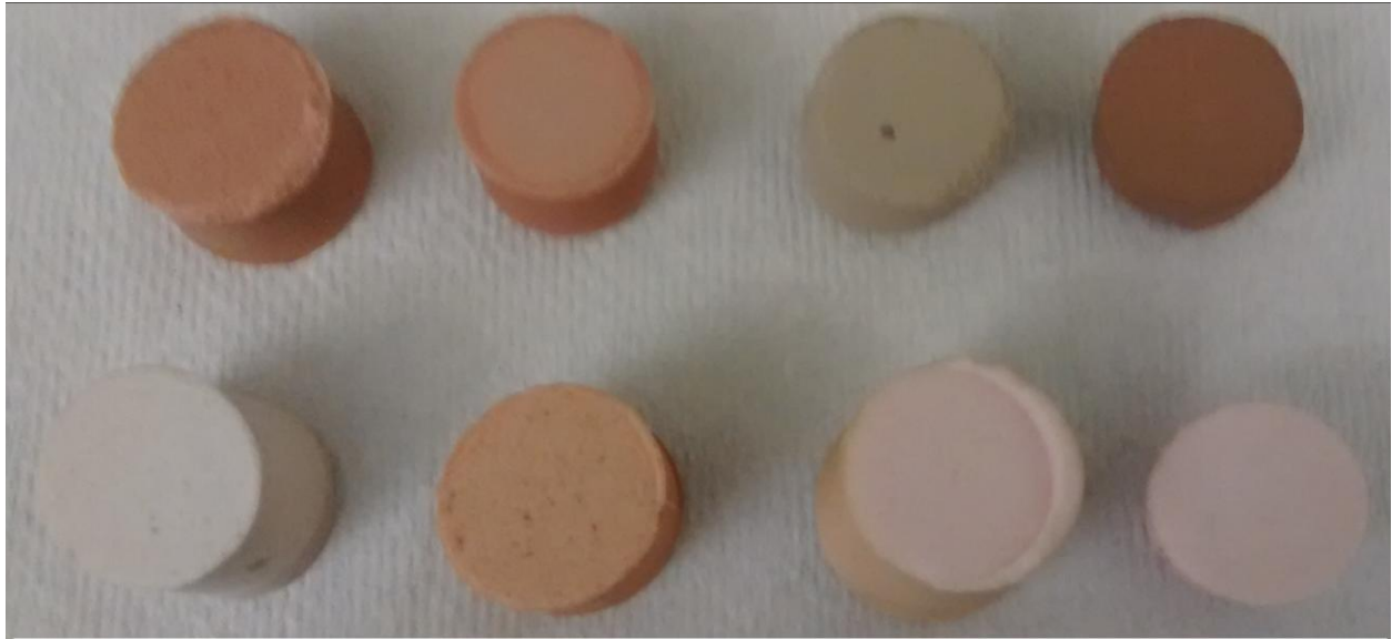
Figure 5-7: Compressed samples at the eight different depths of Rocanville potash mine.
