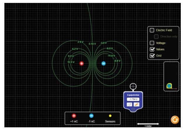
Try to have the equipotential lines equally spaced in voltage. Then, use an E-Field Sensor to measure the electric field at a few points while looking at the relationship between the electric field and the equipotential lines.
