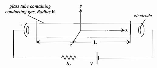
The current spreads out from the electrodes, but remains confined within the tube. For a tube that is much longer than its diameter, away from the electrodes  $\left(-\frac{L}{2} \le X \le + \frac{L}{2}\right)$ , the current density will be radially symmetric, but more concentrated at the centre. As a crude model, consider a *conventional current* density given by:
