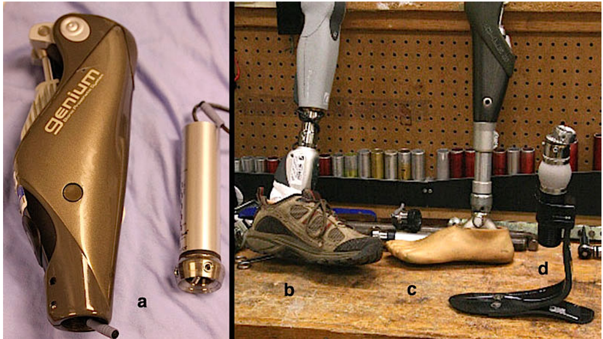
Figure 4-2: An example of lower-limb electromechanical and mechanical prostheses, including a) disassembled microprocessor-controlled robotic prosthetic leg, and a clinical prosthetics workbench demonstrating b) an assembled prosthetic knee and ankle robot; c) an assembled knee-only prosthesis; and d) a purely mechanical, non-robotic prosthetic foot.
